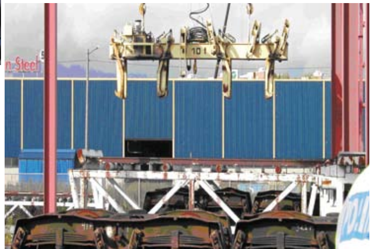
Crane at Port of Turku to change rail gauge from Finnish wide gauge to European mainland normal gauge, Photo: TuTech
